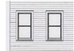
Replacement 1 over 1: Poor selection. No muntins reduces character of original windows.
