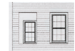
Replacement: Poor selection. Wrong size and proportion.
